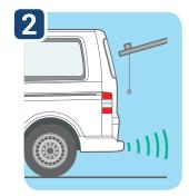
Parking sensor systems rely on either ultrasonic or electromagnetic waves to detect obstacles, so it may not work if the sensors are dirty or out of alignment. Small objects or objects that are too far above or below the sensors, kerbs (I) or garage doors (2) might not be picked up by the system.
